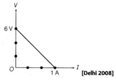
**Ans.** Terminal potential difference across a cell can be obtained by subtracting potential drop across internal resistance of the cell from the emf of the cell.
