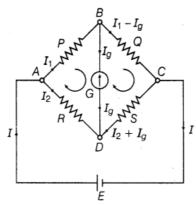
32.Draw a circuit diagram for a Wheatstone bridge. Explain briefly how the balance condition for the galvanometer to give null deflection provides a practical method for the determination of an unknown resistance? [Delhi 2008] Ans.
