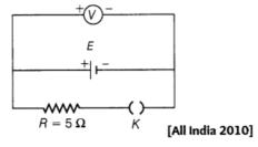
**Ans.** The high resistance voltmeter means that no current with flow through it hence, there is no potential difference across it. So, the reading shown by the high resistance voltmeter can be taken as the emf of the cell.
