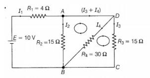
According to figure  $15\Omega$ ,  $30\Omega$  and  $15\Omega$  are in parallel, their equivalent resistance ( $R_{\rm eq}$ ) is
