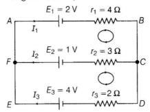
At F, applying junction rule  $I_3 = I_1 + I_2 \qquad ...(i)$
