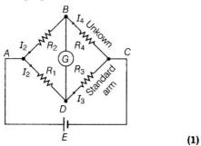
$R_1$ ,  $R_2$ ,  $R_3$  and  $R_4$  are the four resistances. Galvanometer (G) has a current  $I_g$  flowing through it at balanced condition,
